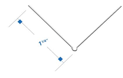
It is used to protect the corners of gypsum board walls and all edges that are exposed to damage from blows (around doors, windows or niches) or any damage due to use.
