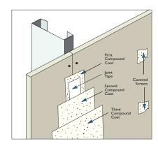
thoroughly dry and keep proper ventilation in the work area to eliminate excess moisture (Gypsum Association GA-236. We recommend the application of a drywall primer to balance the absorption of paint between the surface of the compound and the drywall. Joint compounds and finishing products have a 9 months warranty, effective from the date of manufacture, and when stored under normal conditions, and away from environmental moisture. Do not stow more than two platforms high.
