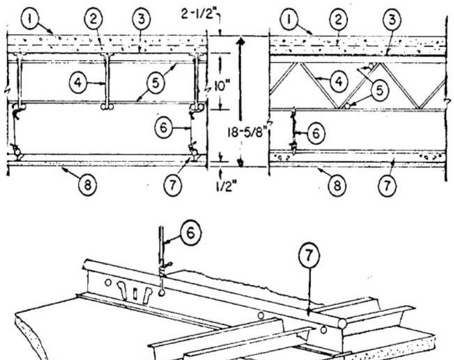
1. **Normal-Weight Concrete** — Carbonate or siliceous aggregate, 152 + or - 3 pcf unit weight, 4500 psi compressive strength.
