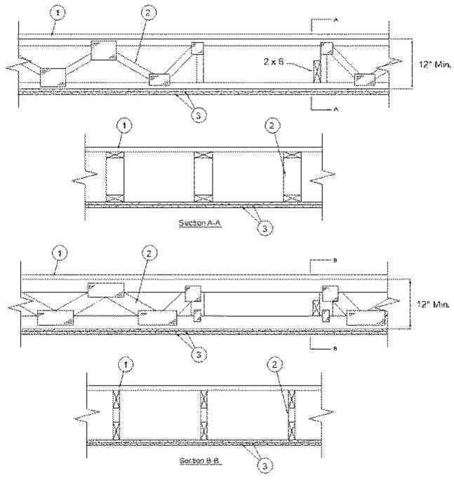
1. Flooring System — The flooring system shall consist of one of the following:
