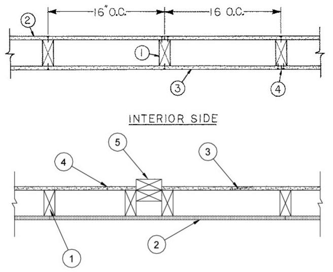
1. Wood Studs — Nominal 2 by 4 in. spaced 16 in. on center, effectively cross braced at mid-height and fire stopped at top and bottom.
