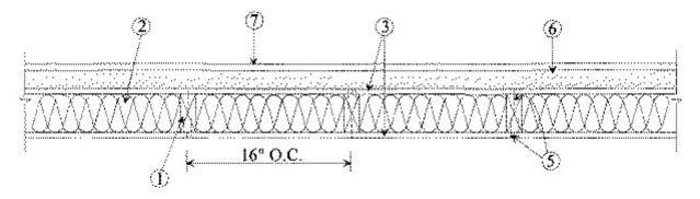
1. Wood Studs – Nom 2 x 4 in. spaced 16 in. OC. Cross braced at midheight and effectively firestopped at top and bottom of wall.
