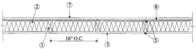
1. Wood Studs — Nom 2 by 4 in. spaced 16 in. OC. Cross braced at midheight and effectively firestopped at top and bottom of wall.
