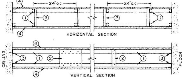
1. **Studs** — Channel shaped, min. 1 5/8 in. depth. Fabricated from No. 25 MSG galv steel. Studs to be cut 1/4 in. less than assembly height.
