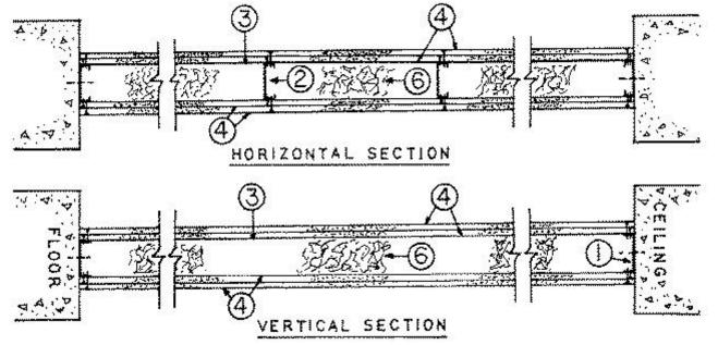
1. Floor and Ceiling Runners — Channel shaped 1/2 in. deep by min 3-5/8 in. wide, No. 25 gauge painted or galvanized steel. Min. No. 18 MSG for the 4 hour rating. Secured with 3/4 in. long concrete fasteners spaced 18 in. OC. For the 1 hour rating, width may be reduced to 2-1/2 in. to accommodate the 2-1/2 in. wide studs.
