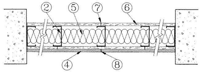
1. **Steel Floor and Ceiling Tracks** — Top and bottom tracks of wall assemblies shall consist of steel members, min No. 20 MSG (0.0329 in., min bare metal thickness) steel or min No. 20 GSG (0.036 in. thick) galv steel or No. 20 MSG (0.033 in. thick) primed steel, that provide a sound structural connection between steel studs and to adjacent assemblies such as floors, ceilings, and/or other walls. Attached to floor and ceiling assemblies with steel fasteners spaced not greater than 24 in. O.C.
